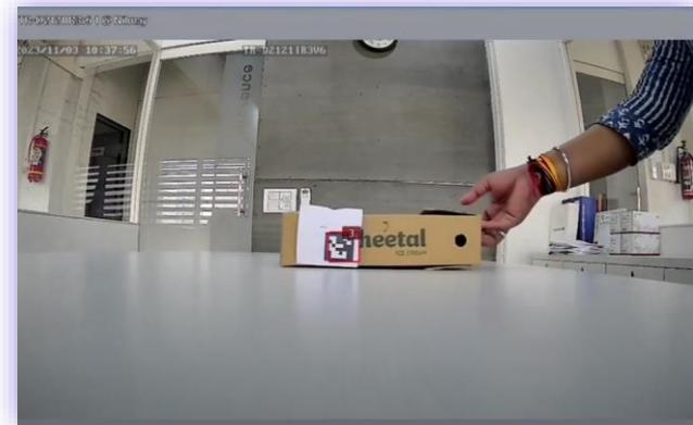
TRASSIR ArUco Detector allows you to recognize ArUco-markers applied to objects. It can be used as an auxiliary tool for accounting in warehouse complexes, logistics distribution centers, production facilities, etc.
